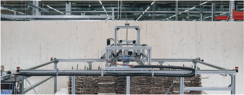
Robotic fabrication of willow components
